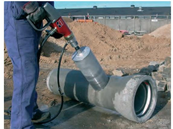
HHCD214 Hand Core Drill
